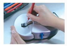
The LM-RondoPlus<sup>™</sup> sharpening machine does not require separate grinding solutions such as water or oil.
